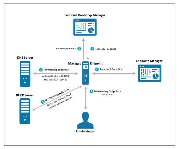
An illustration of PCoIP endpoint discovery process
