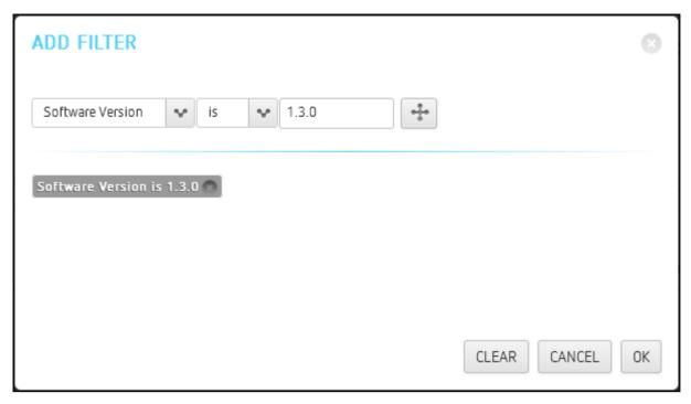
Filter criterion for finding endpoints in recovery mode
