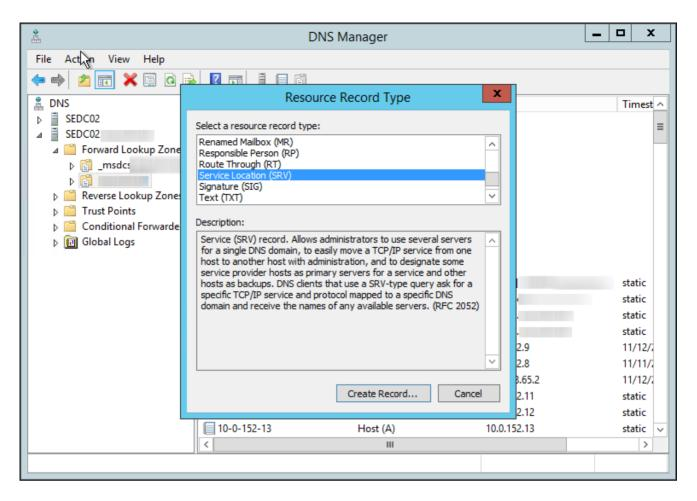
5. Fill in the entries as shown in the following example. Set Service to \_pcoip-bootstrap, Protocol to \_tcp, and *Port number* to 5172, the PCoIP Management Console's default listening port. For *Host offering this service*, enter the PCoIP Management Console's FQDN.
